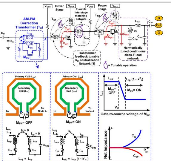
Figure 26.4.2: Schematic of the proposed 2-stage linear PA network incorporating a transformer based AM-PM-distortion correction network.
