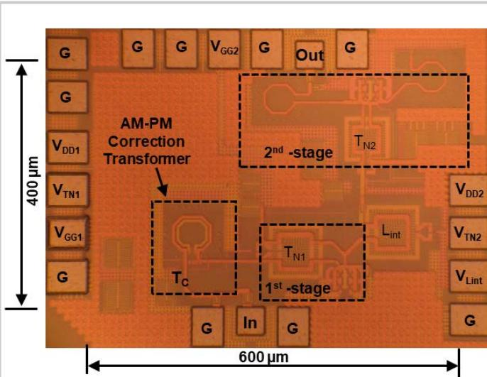
Figure 26.4.7: Die micrograph in a 65nm CMOS technology.
