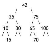
The in-order traversal would print: 10 15 25 30 42 65 70 75 100 The pre-order traversal would print: 42 25 10 15 30 75 65 70 100 The post-order traversal would print: 15 10 30 25 70 65 100 75 42 // The value in each node is not printed until the values of its children are printed
