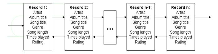
As you can see from the illustration a doubly linked list has a pointer to the next node and the previous node in the list. The first node's previous node pointer is always NULL and the last node's next pointer is always NULL. When you insert and delete
