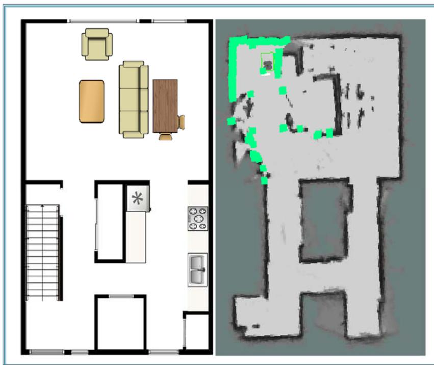
Figure 5. (left) Smart home floorplan. (right) Cartographer-generated home map. Green dots indicate current LiDAR scan.
