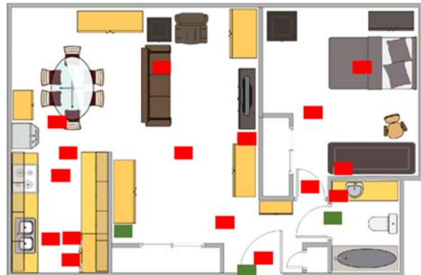
Fig. 10. Smart home floorplan and positions of motion/light sensors (red) and door/temperature sensors (green).
