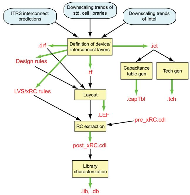
Fig. 2. Design flow of our  $22\text{nm}$  standard cell library.
