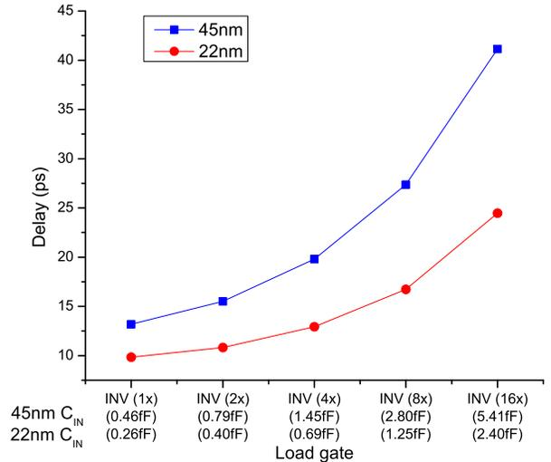
Fig. 4. Delay of a minimum-size inverter driving an  $n \times$  inverter ( $n = 1, 2, 4, 8, 16$ ). Parasitic RC is included. The numbers in the parentheses of the second (or the third) row in the x-axis are the input capacitances of the  $n \times$  inverter.
