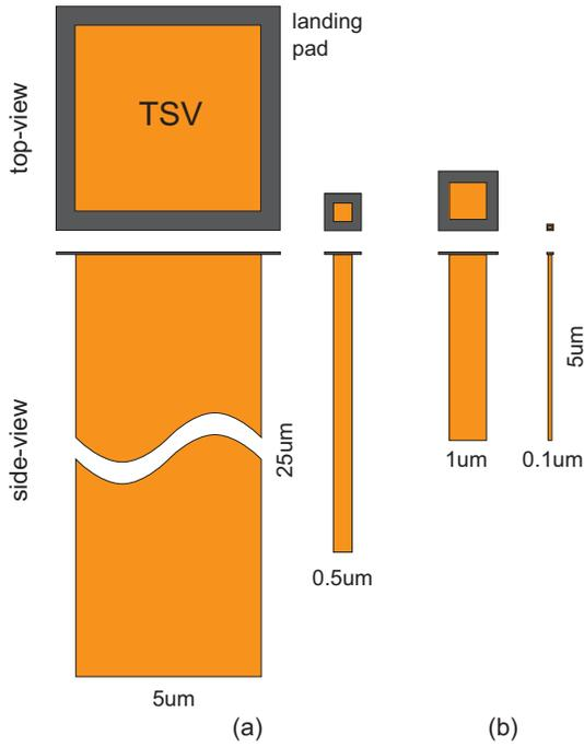
Fig. 6. Size comparison of the 4 TSVs used in our study: (a)  $5\mu\text{m}$  and  $0.5\mu\text{m}$  width used for  $45\text{nm}$  technology, (b)  $1\mu\text{m}$  and  $0.1\mu\text{m}$  width used for  $22\text{nm}$  technology.
