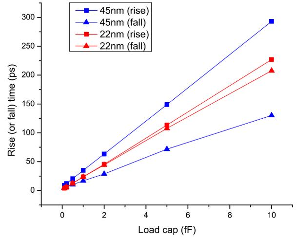
Fig. 3. Comparison of drive strength of a minimum-size inverter driving a load capacitor. Parasitic RC is not included.
