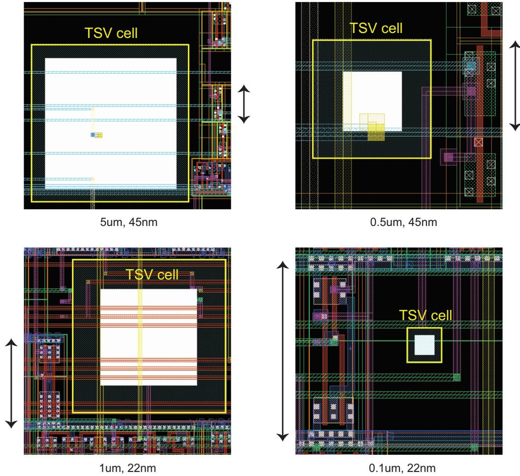
Fig. 7. TSV vs gate size comparison (Cadence Virtuoso GDSII layouts). The TSV cell (= yellow box) includes TSV landing pad and its keep-out zone. The arrow shows the height of the standard cell in each layout.
