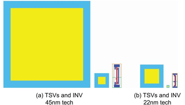
Fig. 1. TSVs and inverters (INV) under two different technologies used in our study (Cadence Virtuoso shot, shown in scale): (a)  $5\mu\text{m}$  and  $0.5\mu\text{m}$  width TSVs and INV under  $45\text{nm}$  technology. (b)  $1\mu\text{m}$  and  $0.1\mu\text{m}$  width TSVs and INV under  $22\text{nm}$  technology.
