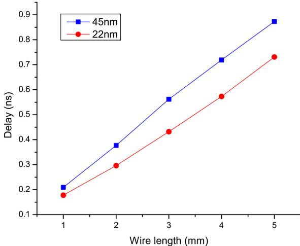
Fig. 5. Delay comparison of buffered global interconnects in 45nm vs 22nm
