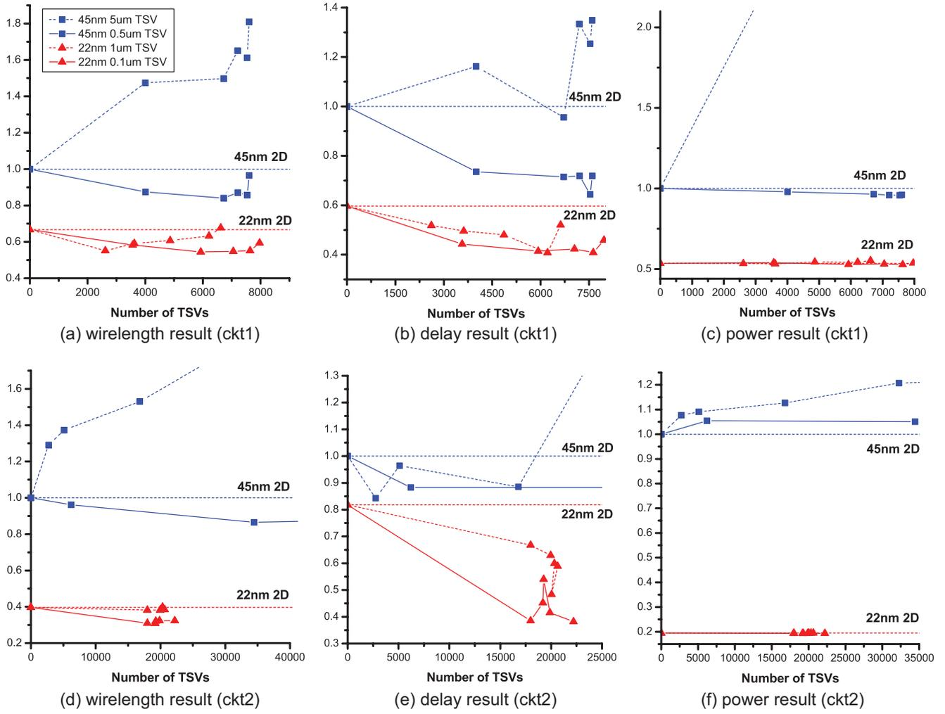
Fig. 8. Wirelength, delay, and power comparison among the full-chip 3D layouts designed with (1) 45nm technology + 5 $\mu$ m width TSV, (2) 45nm technology + 0.5 $\mu$ m width TSV, (3) 22nm technology + 1 $\mu$ m width TSV, and (4) 22nm technology + 0.1 $\mu$ m width TSV.
