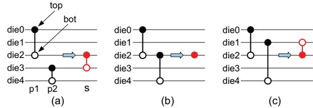
Fig. 5. Die span diagrams. Solid dots are *top* variables and empty dots are *bot* variables. Red spans show *tTop* and *tBot* when we determine the die span of  $s$ . (a)  $t\text{Top} (=2) < t\text{Bot} (=3)$ . (b)  $t\text{Top} (=2) = t\text{Bot} (=2)$ . (c)  $t\text{Top} (=2) > t\text{Bot} (=1)$ .
