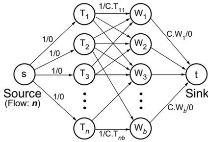
Fig. 6. Global assignment of TSVs to whitespace blocks.  $T_i$  is the  $i$ -th TSV and  $W_j$  is the  $j$ -th whitespace block.  $f/c$  in each edge denotes that  $f$  is the maximum flow capacity, and  $c$  is the cost.  $C.T_{ij}$  is the wirelength when TSV  $T_i$  is assigned to whitespace block  $W_j$ .  $C.W_j$  is the maximum number of available TSV slots in whitespace block  $W_j$ .
