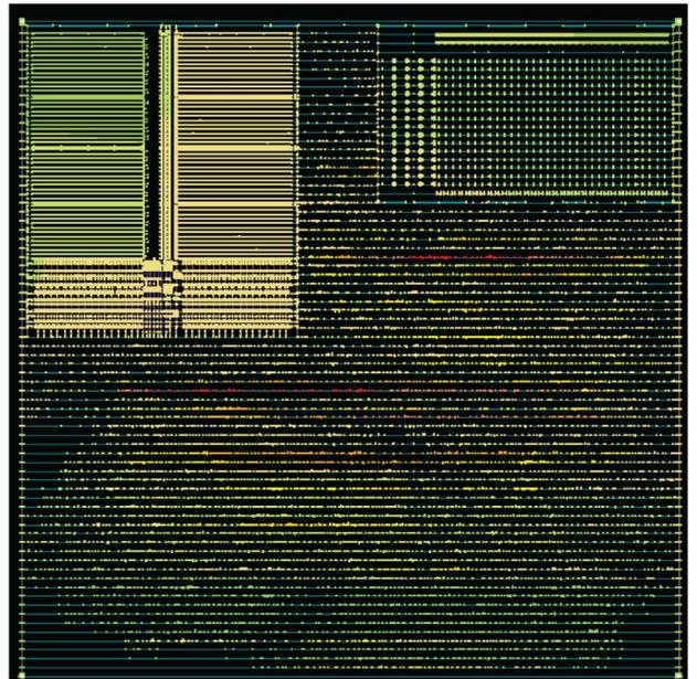
Fig. 12. IR-drop map of a single core. The maximum drop is 60 mV.
