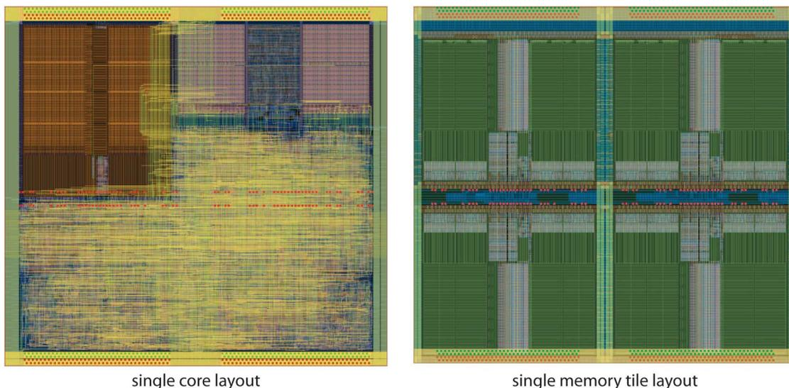
Fig. 5. Single core and memory tile layouts. Red squares in the middle are signal F2F bond pads, and the red/green squares on the top and the bottom are power/ground F2F bond pads.
