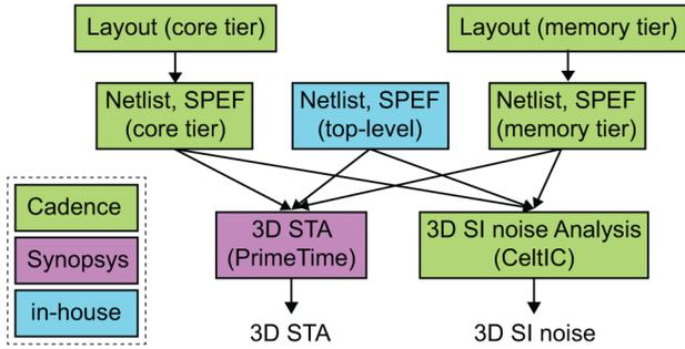
Fig. 9. Our 3D static timing and signal integrity analysis flow.
