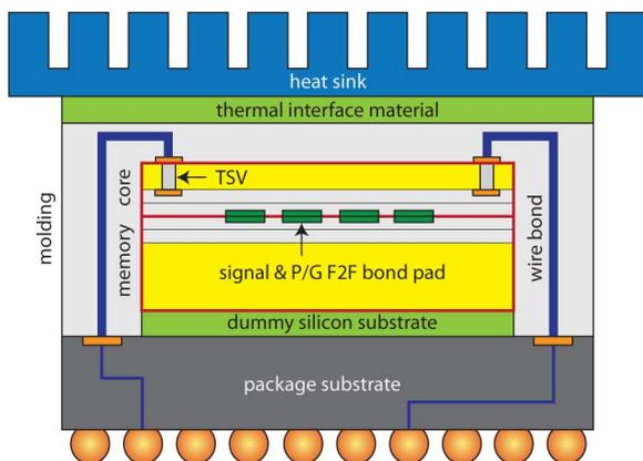
Fig. 3. 3D stacking, TSVs, face-to-face bond pads, and chip-to-package connections.
