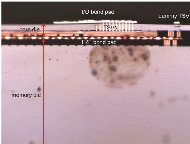
Fig. 17. SEM image of TSVs in an I/O cell, front-side and back-side metal I/O pads, and P/G F2F bond pads.
