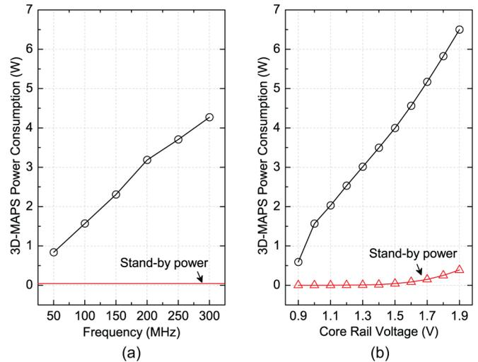
Fig. 18. (a) Frequency vs. power (at 1.5 V), (b) voltage vs. power (at 250 MHz) for the AES encryption benchmark.
