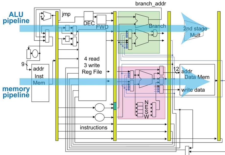
Fig. 2. Details of the single core architecture of 3D-MAPS.
