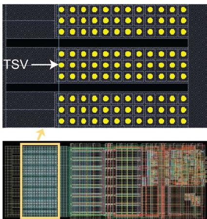
Fig. 8. Redundant TSVs inserted in an I/O pad.
