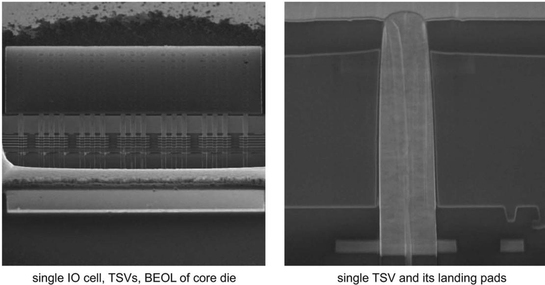
Fig. 16. SEM image of Tezzaron TSVs and face-to-face bond pads.
