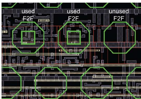
Fig. 6. Used and unused F2F bond pads. The pitch between two adjacent F2F bond pads is 5  $\mu\text{m}$ .
