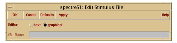
The window shown below opens. This is the window in which the stimulus to the inverter is defined. Observe that the input defined as Vin on the schematic is the entry in this window. You can also find the global input Vdd if you click the Global Sources radio button.
