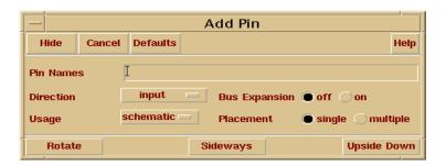
Enter the input pin name as Vin and in the text box, select the input from Direction menu box and press Hide. Place as shown the following window.
