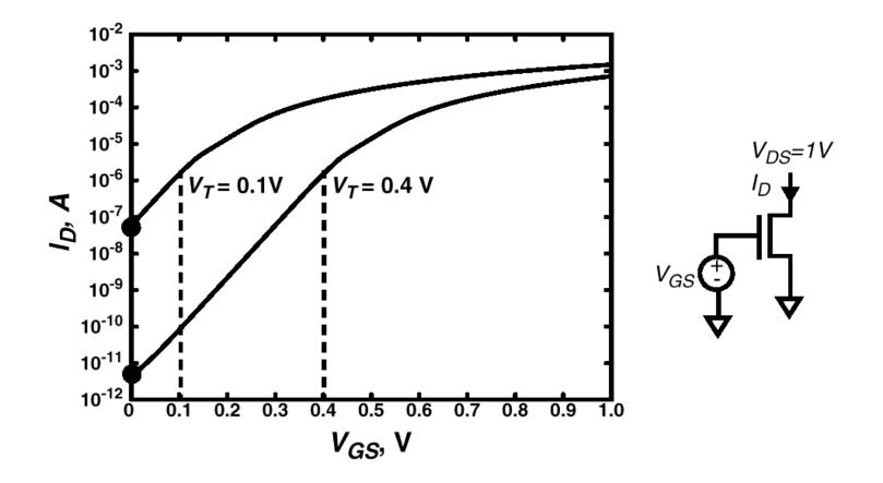
Leakage control is critical for low-voltage operation
