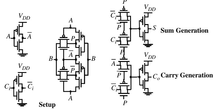
The propagate signal, which is the XOR of inputs A and B, is used to select the true or complementary value of the input carry as the new sum output
