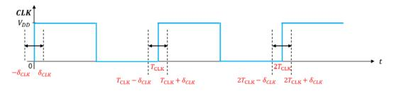
Derive a new setup time and a new hold time constraints (inequalities) that should be satisfied under the variations.
