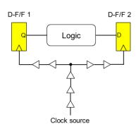
$$T_{s} \leq T_{CLK} - 2\delta_{CLK} - 10\delta_{b} - (T_{logic} + \delta_{logic} + T_{CQ} + \delta_{CQ})$$
