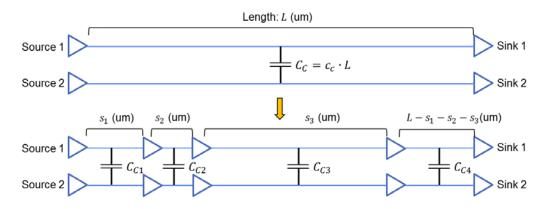
Two nets are routed as shown above. The coupling capacitance between them is  $C_c$ . You are supposed to insert buffers into the nets identically as shown above. All the drivers, sinks, and buffers are of the same type. The following list shows all the parameters and variables you should use:
