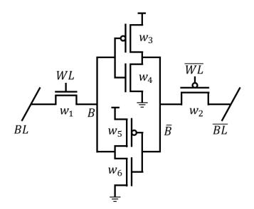
Assume that B = 0 ( $\overline{B} = 1$ ) is stored in the SRAM cell. <u>Derive all inequalities and/or</u> equations for the widths of the six transistors to write 1 to the SRAM cell (in this case, BL and  $\overline{BL}$  are set to 1 and 0, respectively, and WL and  $\overline{WL}$  are set to 1 and 0, respectively, to access the cell and write 1 into the cell). Use the following variables/constants.
