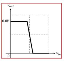
2) Draw a DC characteristic curve ( $V_{in}$  vs.  $V_{out}$ ) when  $V_A = 0.7V$ .
