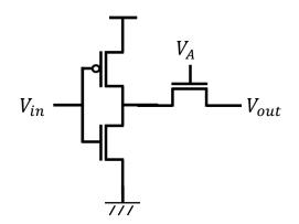
1) Draw a DC characteristic curve ( $V_{in}$  vs.  $V_{out}$ ) when  $V_A = 1V$ .
