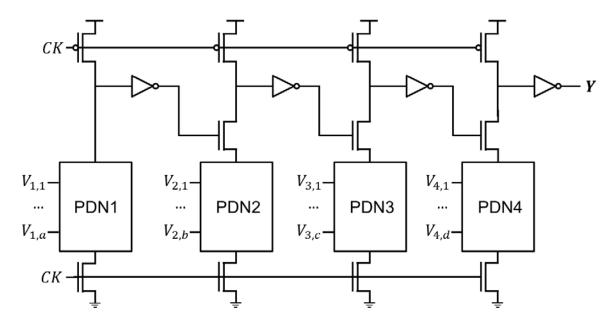
All the inputs are available at time 0 (i.e., <u>the inputs are stable from time 0 until the end</u> <u>of the evaluation</u>). The clock switches from high to low at time 0 for pre-charging and switches from low back to high at time  $t_1$  for evaluation.
