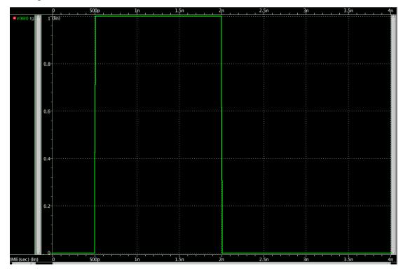
[Submit] Find the rise delay and the fall delay at the output node (Y). Notice that the rise delay is measured by b - a where b is the time when the output reaches 0.9V and a is the time when the input starts switching. The fall time is defined in
