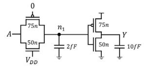
Generate the following input signal and apply it to node A. The transition time is 10ps.
