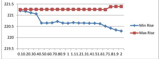
(2) [Process Variation, 20 points] Set the width of the NFET to 50nm (no variation) and that of the PFET to agauss (75n, Xn, 1) where X is (0.1, 0.2, ..., 2.0). Simulate inv.sp for each X and find the min. fall delay and the max. fall delay for each X. [Submit] Plot X vs. min. fall delay. Plot X vs. max. fall delay. Plot X vs. min. rise delay. Plot X vs max. rise delay.
