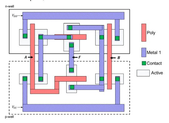
(2) **[Layout, 20 points]** Convert the following layout into a transistor-level schematic. Input: A, B, C. Out: F.
