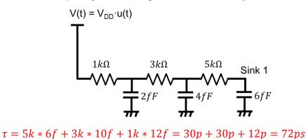
(2) [Elmore Delay, 10 points] Compute the Elmore delays from the source to Sink 1 and Sink 2.
