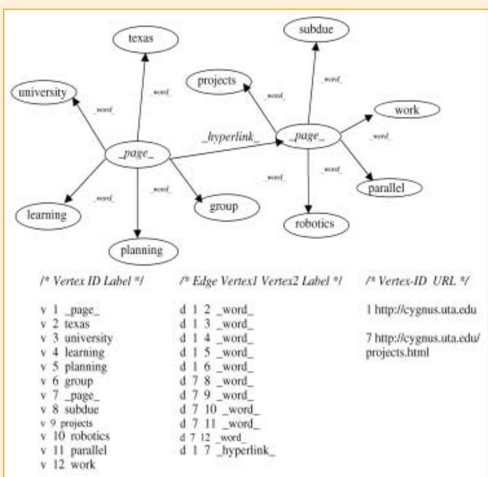
Figure 1. Graph representation of a Web site. A graph is represented as a set of vertices (denoted by v, a vertex id, and a label) and a set of edges (denoted by d for directed edge or u for undirected edge, the source and destination vertex IDs, and a label). Hits are represented by the vertex ID and corresponding URL.
