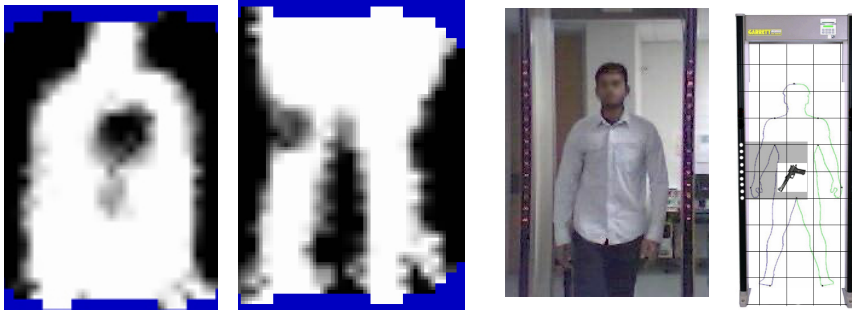
Fig. 1. First from left: Millimeter Wave Image of person carrying suspicious object on their upper chest. Second from left: Millimeter Wave Image of person carrying suspicious object on their right thigh. Third from left: Person walking through Pin-point Metal Detector. Fourth from left: Lights getting illuminated when person carries gun.
