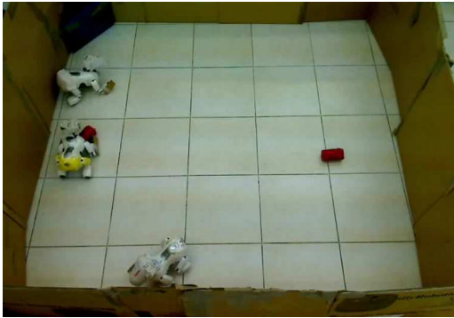
Figure 3: Three Sony AIBO robots executing a foraging task in our laboratory. The goal location is in the top left corner. Every puck collected was taken out of the arena.
