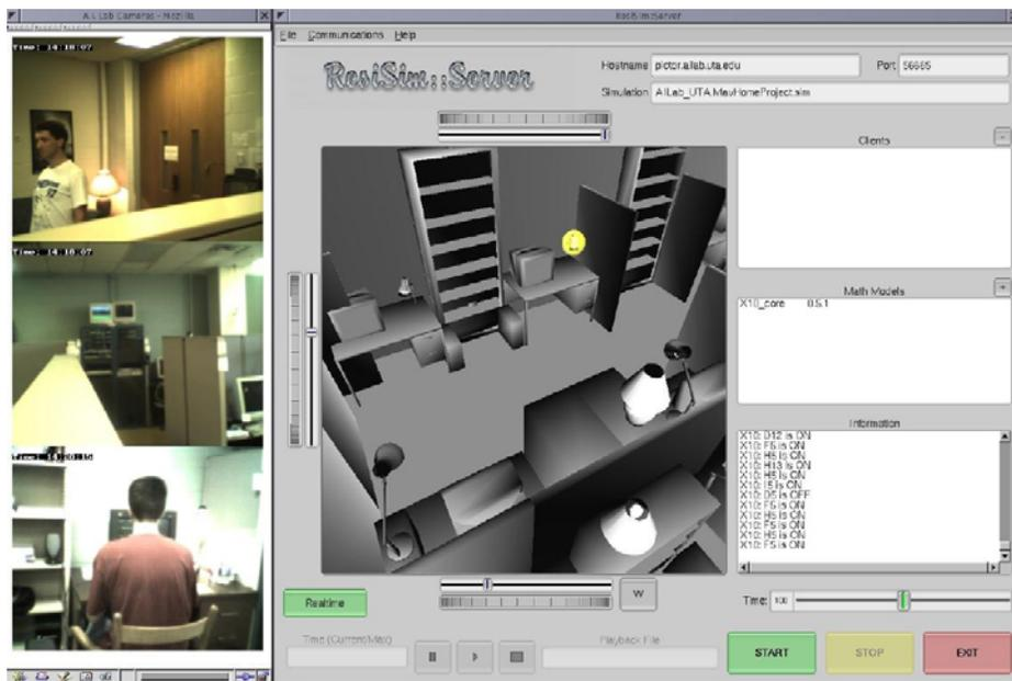
Figure 8. ResiSim update after desk lamp (lower left) is turned on.
