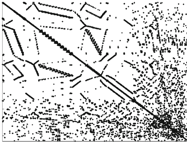
Fig. 9 Sparsity structure of the Hessian of the smallest mesh problem ( gear with n = 2598 )
