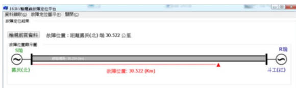
Fig. 6 Graphical display of the fault location estimation result
