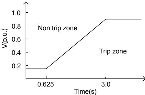
Fig. 3 LVRT voltage-duration profile in FERC order 661
