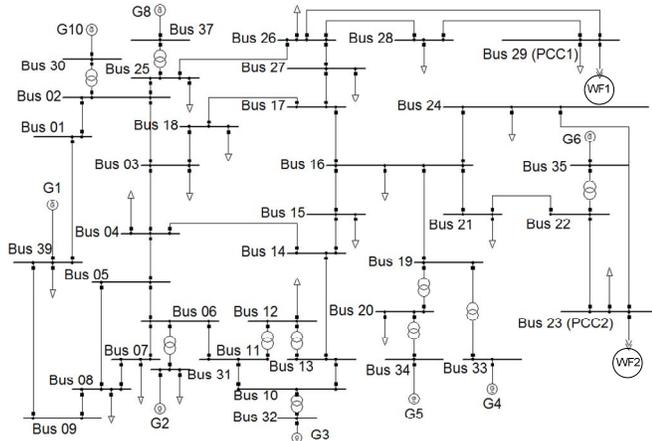
Fig. 4 IEEE 39 bus system with WF connections
