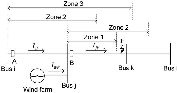
Fig. 2 Portion of power grid with WF connection
