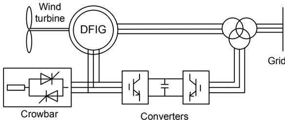
Fig. 1 Typical configuration of DFIG with wind turbine
