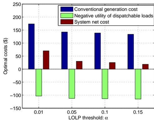
Fig. 3. Optimal costs for different LOLP values.
