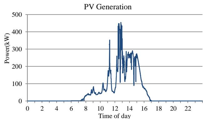
Fig. 2. PV generation power in a cloudy day
