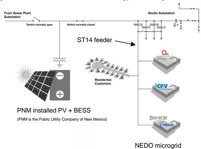
Fig. 1. Feeder ST14 configuration diagram showing the connections to the PV+BESS, the NEDO microgrid, commercial and residential customers.
