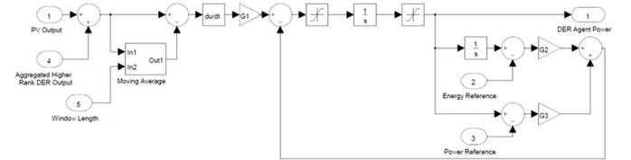
Fig. 5. Smoothing agent power reference block diagram implementing SWMAC method
