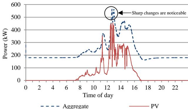
Fig. 7. PV power and the aggregated output. In spite of smoothing, there is still signs of fluctuations in the total output.
