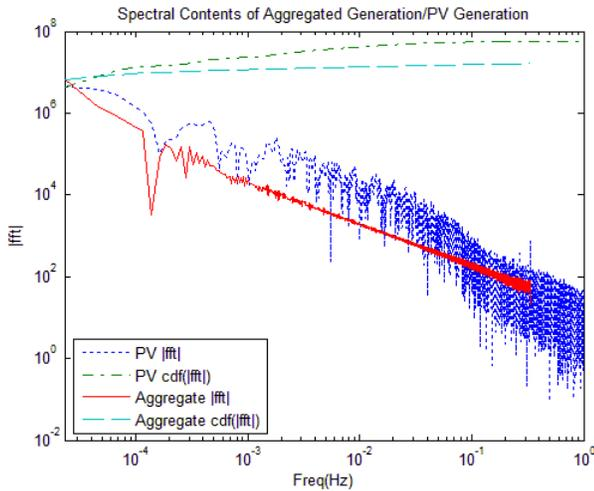
Figure 12. Frequency spectrum of the PV output and the smoothed aggregate power. High energy concentration in the lower frequency range is prevalent.
