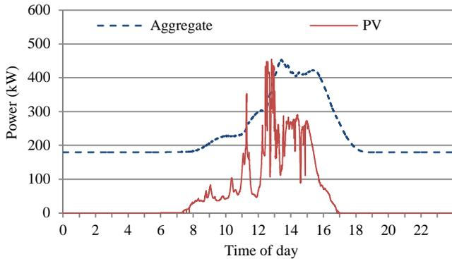
Figure 11. PV power and the aggregated output. Aggregate output is smoother than previous method at the expense of higher energy exchange for the battery
