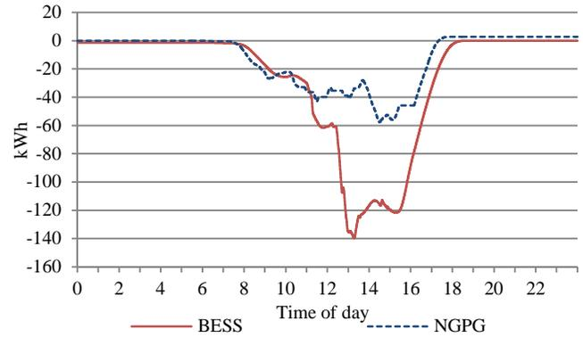
Figure 13. Smoothing energy, exchanged between BESS, NGPG and the grid. Apparently, the storage system is under more stress than RRC method.
