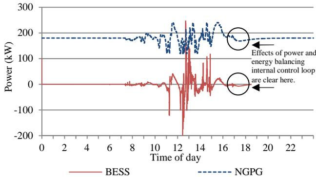
Fig. 6. NGPG and BESS contribution to RRC smoothing. NGPG has tried to follow the PV fluctuations, but due to limited dynamic response and power capabilities, is not able to follow the fast varying portion of the PV. On the other hand, BESS ramps up and down keeping up with PV variations.
