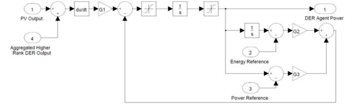
Fig. 4. Smoothing agent power reference controller block diagram implementing RRC method
