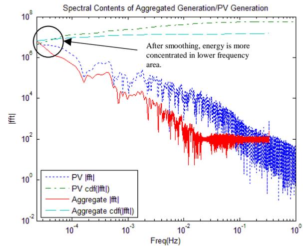
Fig. 8. Frequency spectrum of the PV output and the smoothed aggregate power. Concentration of the smoothed signal around lower frequencies is noteworthy.
