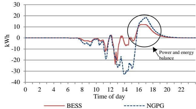
Fig. 9. Smoothing energy, exchanged between BESS, NGPG and the grid.
