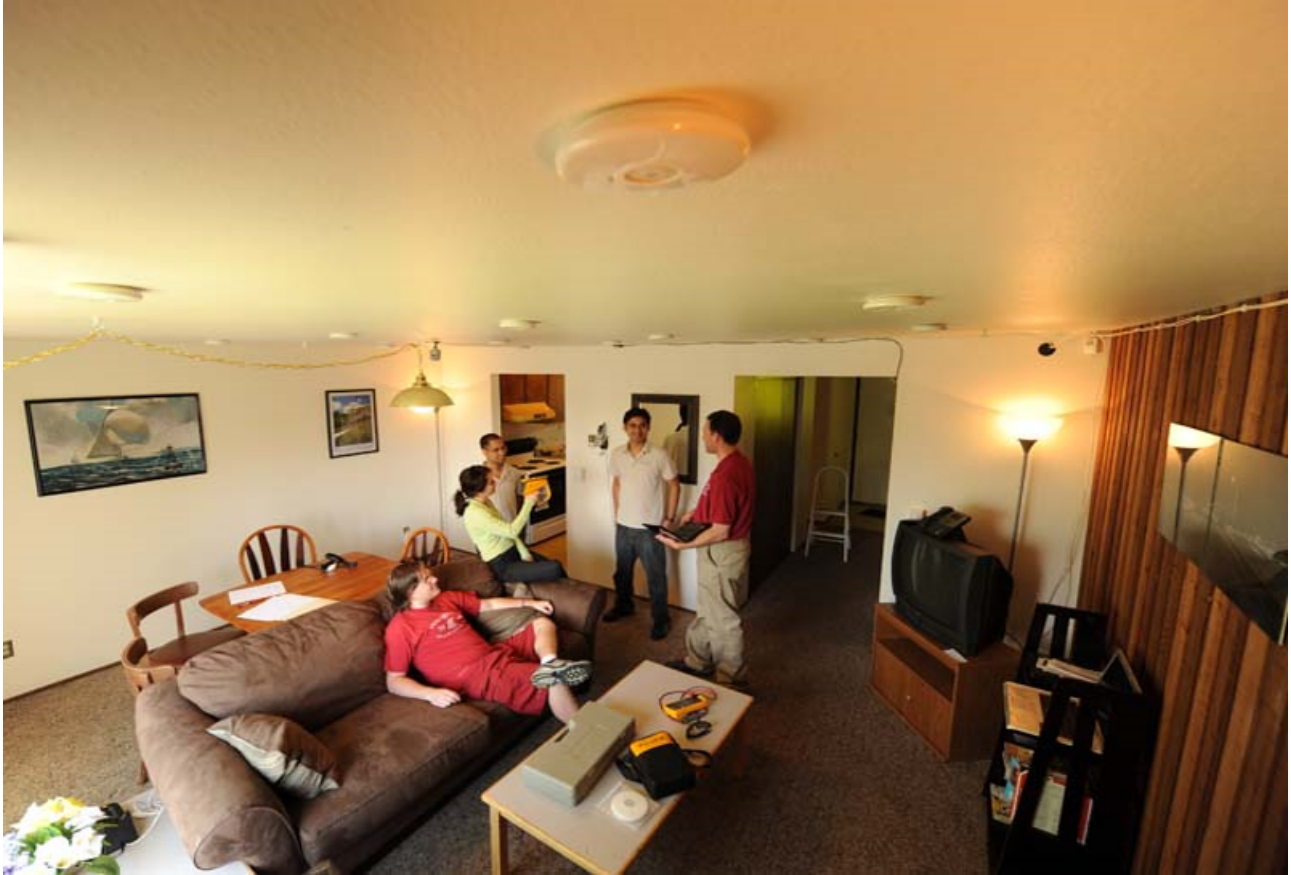
Figure 6.1: A CASAS smart home testbed. Wireless ZigBee passive infrared motion detectors are attached to the ceiling, including top center.
