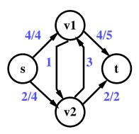
$$c_f(s, v_2) = c(s, v_2) - f(s, v_2) = 4 - 2 = 2$$
