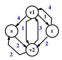
If there is a path from s to t in the residual network, then it is an augmenting path and indicates where flow can increase.
