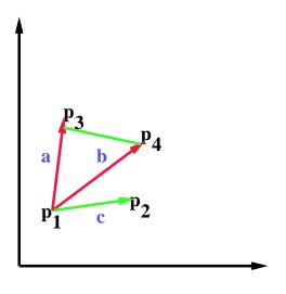
$$\begin{array}{l} \vec{a} \times \vec{c} < 0 \\ \vec{b} \times \vec{c} < 0 \end{array}$$
