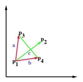
$$\begin{array}{l} \vec{a} \times \vec{c} < 0 \\ \vec{b} \times \vec{c} > 0 \end{array}$$
