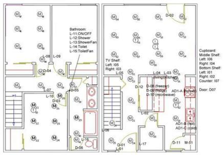
Figure 2: Three-bedroom smart apartment used for data collection (Sensors: motion (M), temperature (T), water (W), burner (B), telephone (P) and item (I)).
