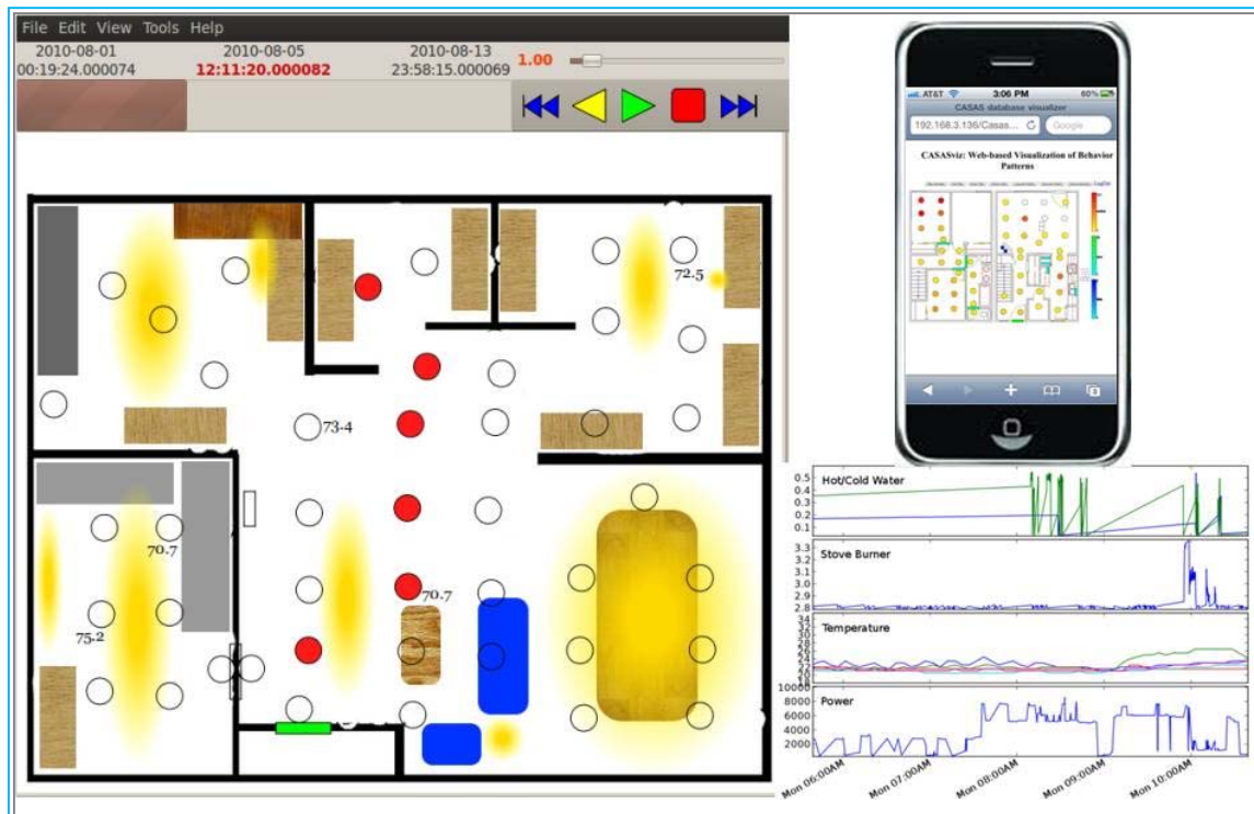
Figure 5. Snapshot of CASAS activity visualizer. The visualizer renders sensor events on a computer or mobile device while plotting usage of resources such as electricity.
