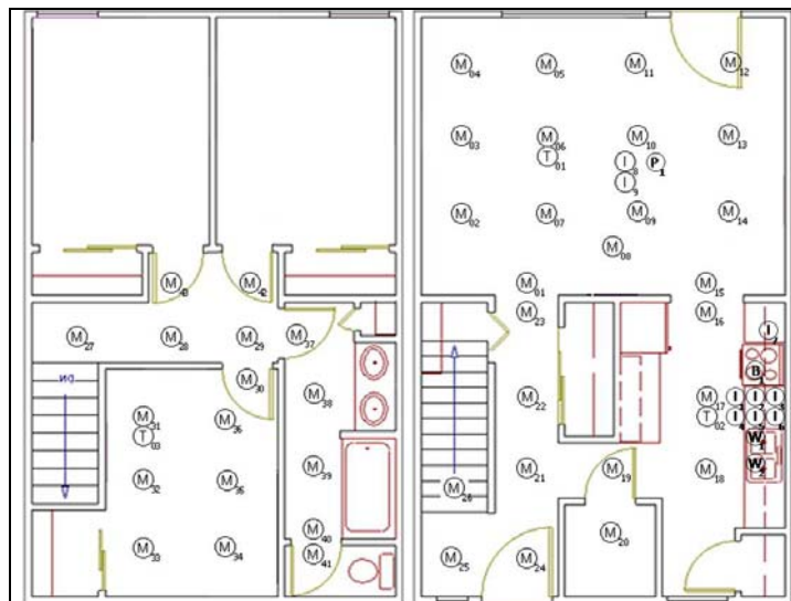
Figure 3. The CASAS apartment. Circles indicate the positions of motion (M), temperature (T), and item (I) sensors throughout the environment.
