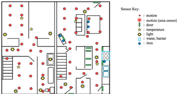
Figure 7. The layout of the CASAS smart home test bed that was used to test smart home features. Both the activity recognition and activity prediction features are capable of incorporating live smart home test bed sensor data.
