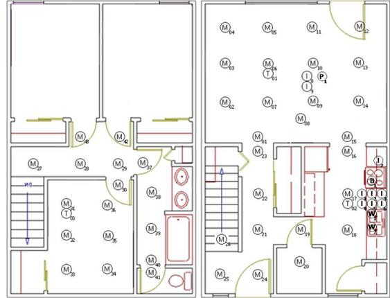
Figure 2. Diagram of our first living environment and sensor locations. Circles with M inside them represent a ceiling-mounted motion detector, T’s are temperature sensors, and I are item sensors. The subscript refers to its local id number.
