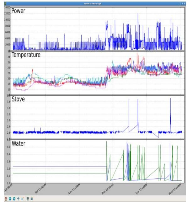
Figure 2. Project CASAS: Physical test bed for smart environment data collection. The bottom portion of the figure displays power usage as well as readings for temperature, stove use, and water use while sensor events are generated (shown as red circles) in the testbed environment. The power data was collected by a simple power meter device.
