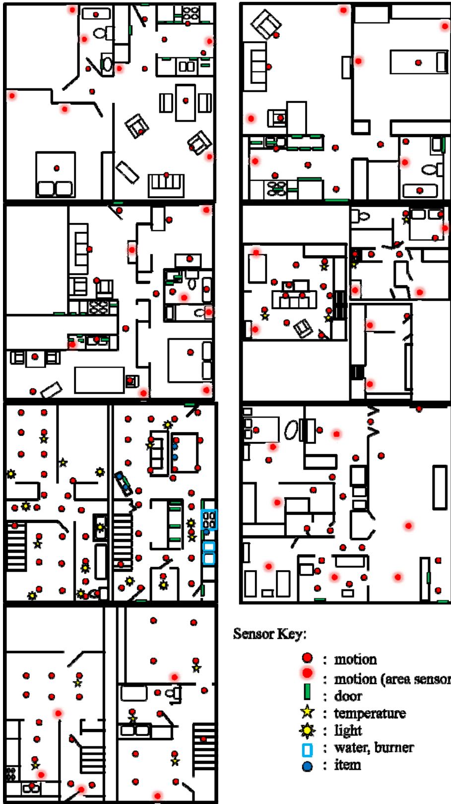
Figure 1. Sensor layout for the seven CASAS smart environment testbeds: Bosch1 (first row left), Bosch2 (first row right), Bosch3 (second row left), Cairo (second row right), Kyoto (third row left), Milan (third row right), and Tulum (bottom row).
