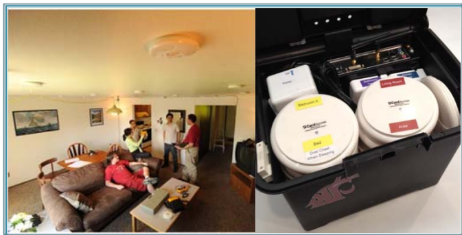
Figure 1. (left) Motion/light sensors and door/temperature sensors are installed in a smart home; (right) the SHiB kit includes sensors, computer, and networking equipment.
