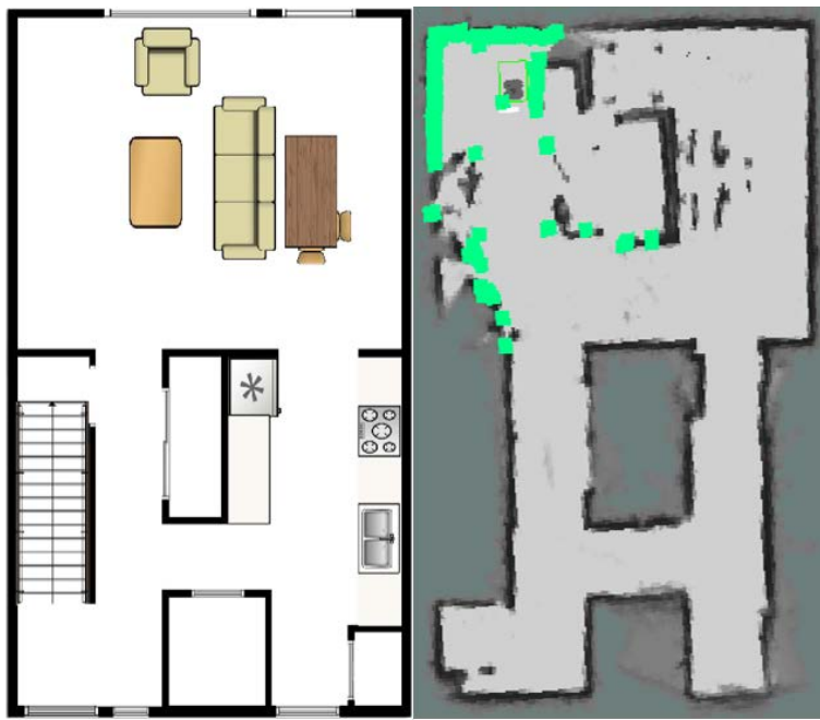
Figure 7: Actual layout for bottom floor of smart home with added furniture from Figure 2 (left) and RAS-learned map of navigable smart home regions (right). In the robot map, green dots highlight the current LiDAR scan and the dark green rectangle represents the robot’s bounding box.
