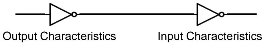
Low noise margin =  $NM_L = |V_{IL,max} - V_{OL,max}|$
