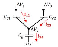
[**Submit**] Represent  $\Delta V_2$  as a function of  $\Delta V_1$ ,  $\Delta V_3$ ,  $C_{c1}$ ,  $C_{c2}$ , and  $C_g$ .
