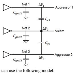
To compute  $\Delta V_2$ , we can use the following model:
