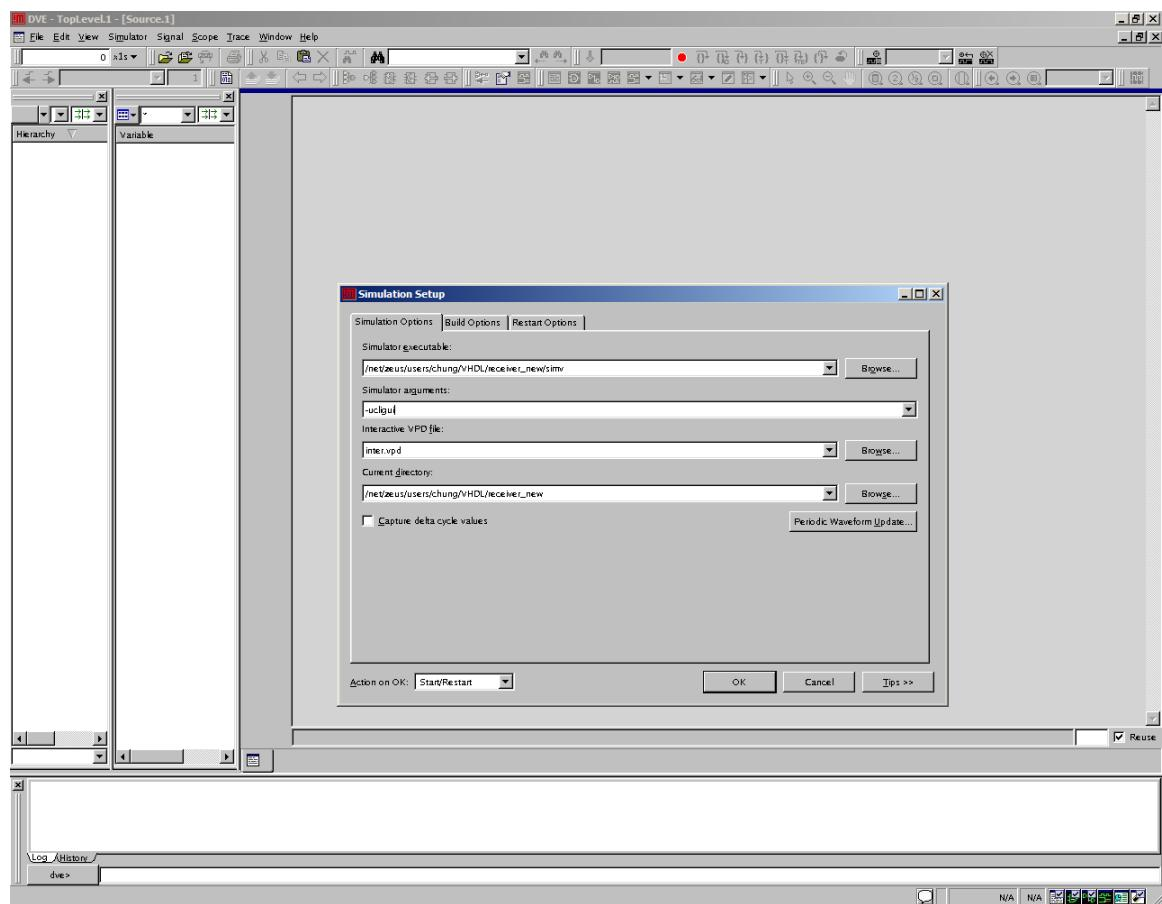
c. This opens up your design with the list of signals on the left panel. Select the signals that you want to observe in your waveform, right click and choose “Add to Waves → New Wave View” from the menu. For an example, see the screenshot below.
