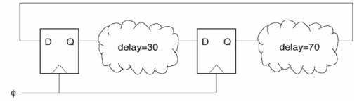
(b) Suppose you are designing a datapath using custom-layout techniques. Your data flows from left to right, as shown in the following two diagrams. In the first diagram, the clock is driven by a driver on the left side of the chip, and the clock propagates from left to right. In the second diagram, the clock is driven by a driver on the right of the chip, and the clock propagates from the right to the left. Which design is safer? [3]
