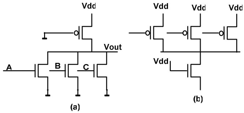
(b) What is the logic function (Y) computed by the following circuit?
