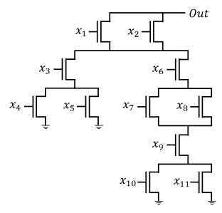
(4) [Design and transistor sizing, 20 points] Draw a PFET network for the static CMOS gate shown above (in Problem 3). Use only 11 PFETs. Size the transistors. Timing constraint:  $\tau = R_n C_L$  where  $R_n$  is the resistance of a 1X NFET and  $C_L$  is a load cap.  $\mu_n = 3\mu_p$ . The total width should be less than 120X.
