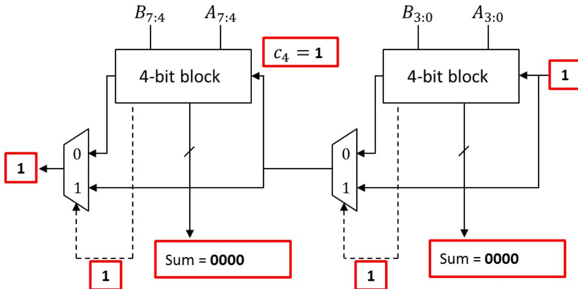
(3) [Adder, 10 points] Add the following three numbers using the conditional sum adder shown below. A=11101110, B=01111001, Cin=1 (Fill in the blank boxes).
