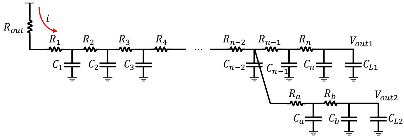
$$\begin{aligned}\tau(V_{out1}) = & R_n(C_n + C_{L1}) + R_{n-1}(C_{n-1} + C_n + C_{L1}) + \\& R_{n-2}(C_{n-2} + C_{n-1} + C_n + C_{L1} + C_a + C_b + C_{L2}) + \\& \dots + R_3(C_3 + \dots + C_n + C_{L1} + C_a + C_b + C_{L2}) + \\R_2(C_2 + \dots + C_n + C_{L1} + C_a + C_b + C_{L2}) + & R_1(C_1 + \dots + C_n + C_{L1} + C_a + C_b + C_{L2}) + \\R_{out}(C_1 + \dots + C_n + C_{L1} + C_a + C_b + C_{L2})\end{aligned}$$
