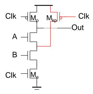
Precharge internal nodes using a clock-driven transistor (at the cost of increased area and power)
