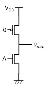
$$\frac{\beta_n}{2} \left[ 2(V_{DD} - V_{tn})V_{OL} - V_{OL}^2 \right] = \frac{\beta_p}{2} (V_{DD} - |V_{tp}|)^2$$
