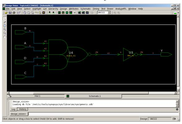
Open test\_syn.v in a text editor. This shows the synthesized netlist. You will see that it uses an AOI22\_X1 cell (implementing  $\overline{A1 \cdot A2 + B1 \cdot B2}$ ) and an inverter cell.
