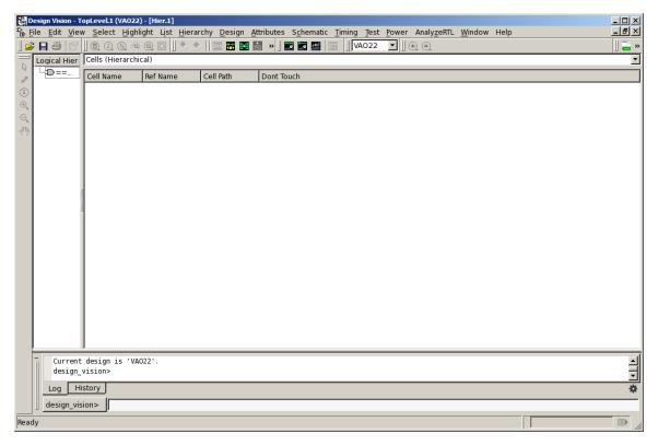
Click the gate symbol under "Logical Hierarchy". Then, click Schematic  $\rightarrow$  New Schematic View.
