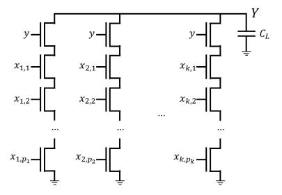
The width of the transistors in the i-th column:  $w_i$
